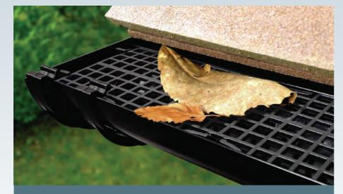
A popular addition to any system is **Gutter Guard**. Designed to prevent leaves and other debris from blocking outlets and down pipes, Gutter Guard simply sits in the gutter with no need for screws or brackets. It can be used with any PVC-U guttering between 100 and 115mm wide and is easily trimmed to size or clipped together to form a continuous run. The use of cable ties may be required.
